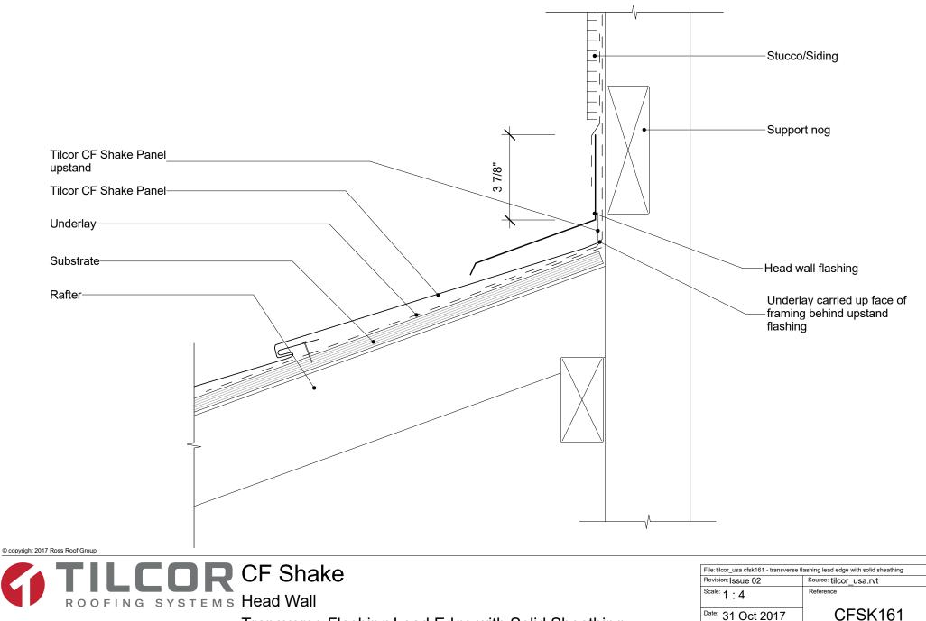
Transverse Flashing Lead Edge with Solid Sheathing
