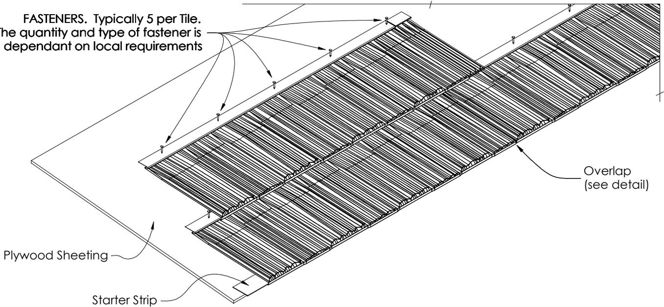
Figure 11.2 Fastening Detail
