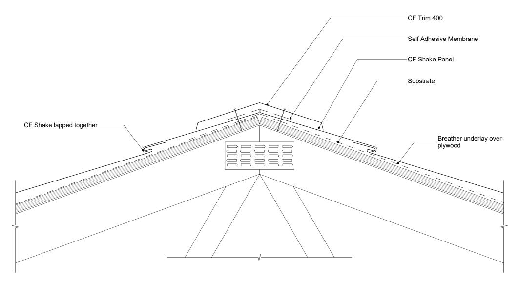
Ceopyright 2017 Ross Roof Group TILCOR CF Shake ROOFING SYSTEMS Ridge Detail
