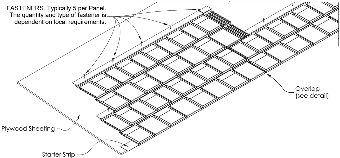
Figure 12.2 Fastening Detail
