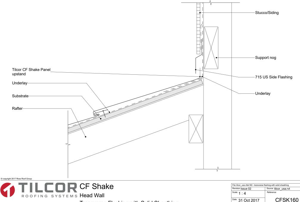
Transverse Flashing with Solid Sheathing
