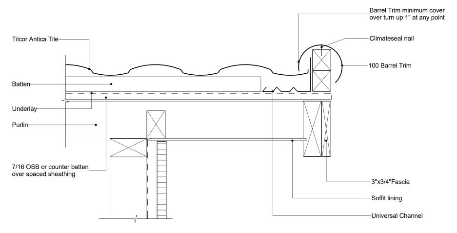
\* Barge board must project at least to top of tile batten
