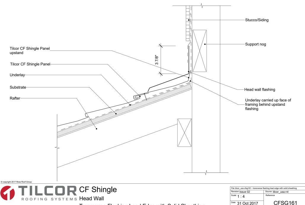
Transverse Flashing Lead Edge with Solid Sheathing
